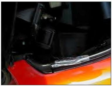
Any water should drain down the gully to the drain hole just behind the seat belt mounting. The start and end points of the gully are marked by the yellow circles in the pictures below.
