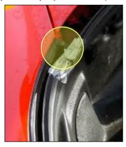
When you close the tonneau cover it will locate in the top of the gasket and form a waterproof seal.
